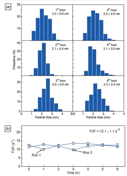
Fig. 5 (a) Particle size distributions of the PdNP sample assessed hourly during a 6 hour production run, highlighting the consistency in the particle size for prolonged operation. (b) Catalytic activities of PdNPs in terms of the turnover frequency (TOF) for samples assessed hourly from two separate 6 hour nanoparticle production runs, highlighting the consistency in the quality of PdNPs over prolonged operation (see the ESI† for further information).
