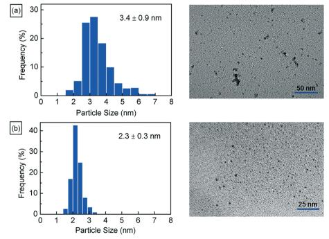
Fig. 3 (a) Particle size distribution and TEM image for batch-synthesized PdNPs with an average size of 3.4 ± 0.9 nm. (b) Particle size distribution and TEM image of flow-synthesized PdNPs with an average size of 2.3 ± 0.3 nm, highlighting smaller mean size and narrower particle size distribution compared to those produced using the small-scale batch reactor.
