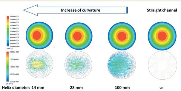
Fig. 10 Fluid dynamic simulation results of the effect of helix diameter on the formation of secondary transverse flows with an inlet velocity of 0.1 m s<sup>-1</sup>. The upper row shows the cross section velocity magnitude contour and the bottom row shows the corresponding cross section velocity vectors
