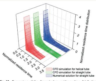
Fig. 12 Comparison of the dimensionless residence time distribution function in a straight and a helical reactor with a helix diameter of 14
