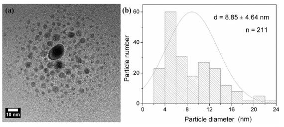
Fig. 9 (a) TEM images and (b) particle size distributions of AgNPs synthesized in helical tubular microreactors with a length of 130 cm, a helix diameter of 100 mm and a helix pitch of  $1/\pi$  mm.
