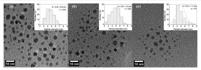
Fig. 3 TEM images and particle size distributions of AqNPs synthesized in helical tubular microreactors with lengths of (a) 60 cm, (b) 95 cm, and (c) 130 cm. Conditions: helix diameter: 14 mm, helix pitch:  $1/\pi$  mm, and total flow rate: 0.7 mL min<sup>-1</sup> with an AgNO<sub>3</sub>/NaBH<sub>4</sub> molar ratio of 1:6.
