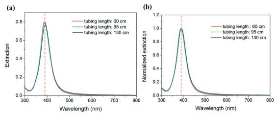
Fig. 4 (a) UV-vis extinction spectra and (b) normalized extinction spectra for AqNPs synthesized in helical tubular microreactors with different tubing lengths. Conditions: helix diameter: 14 mm, helix pitch:  $1/\pi$  mm, and total flow rate: 0.7 mL min<sup>-1</sup> with an AqNO<sub>3</sub>/NaBH<sub>4</sub> molar ratio of 1:6.
