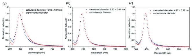
Fig. 17 Fitting of the experimental UV-vis spectra of silver nanoparticles synthesized in helical reactors with varying total flow rates of (a) 0.15 ml  $min^{-1}$ , (b) 0.5 ml  $min^{-1}$  and (c) 0.7 ml  $min^{-1}$ , a length of 130 cm, a helix diameter of 14 mm, and a helix diameter of  $1/\pi$  mm with an AgNO<sub>3</sub>/NaBH<sub>4</sub> molar ratio of 1:6 using the Mie model.
