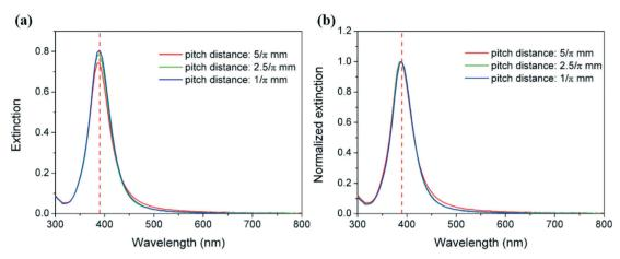
Fig. 13 (a) UV-vis extinction spectra and (b) normalized extinction spectra for AgNPs synthesized in helical tubular microreactors with different pitch distances. Conditions: reactor length: 60 cm, helix diameter: 14 mm, and total flow rate: 0.7 mL min<sup>-1</sup> with an AgNO<sub>3</sub>/NaBH<sub>4</sub> molar ratio of 1:6.
