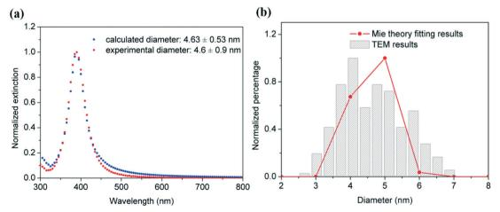
Fig. 6 (a) Comparison of the experimental UV-vis spectra of silver nanoparticles synthesized in helical tubular microreactors (length: 60 cm, helix diameter: 14 mm and helix pitch:  $1/\pi$  mm, total flow rate: 0.7 mL min<sup>-1</sup> with an AqNO<sub>3</sub>/NaBH<sub>4</sub> molar ratio of 1:6) and the predicted one using the Mie model. (b) Comparison of particle diameter distributions obtained from the Mie model and TEM images.
