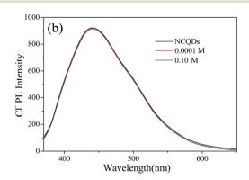
Fig. 6 (a) Relative fluorescence intensities of NCQDs in the presence of various metal ions at the concentration of 1 mM. The excitation wavelength is 360 nm. (b) FL spectra of NCQDs in the presence of 0.0001 and 0.1 M  $Cl^-$ .
