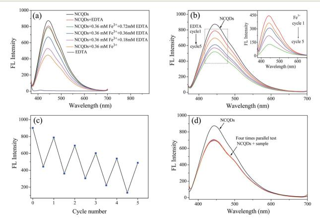
Fig. 9 (a) The fluorescence recovery of NCQDs by EDTA. (b) The reversible fluorescence spectra of NCQDs when alternately added EDTA and Fe<sup>3+</sup> (the inset). (c) The reversible switching cycles. (d) The fluorescence guenching of leaching solution of iron ore tailings to NCQDs.
