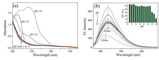
Fig. 5 (a) UV-vis absorption spectra of NCQDs at different pH values. (b) Fluorescence emission spectra of NCQDs at different pH values. Inset shows QYs at different pH values.
