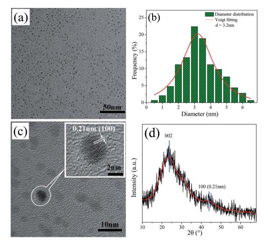
Fig. 2 (a) TEM images, (b) the size distributions histogram, (c) HRTEM images, and (d) XRD pattern of NCQDs. Inset of (c) shows enlarged image of HRTEM.
