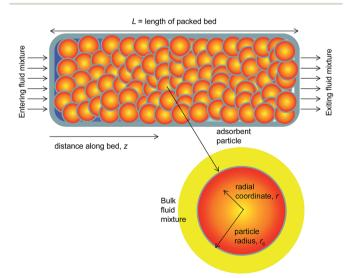
Fig. 2 Schematic of fixed bed adsorber filled with adsorbent particles of radius  $r_{\rm c}$ .
