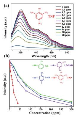
Fig. 3 (a) Emission spectra of 1 titrated with TNP in DMF for about 2 minutes. (b) Relationship between the emission intensities and the corresponding concentrations for NB (green), I-NB (blue), 1,3-DNB (violet) and TNP (red).
