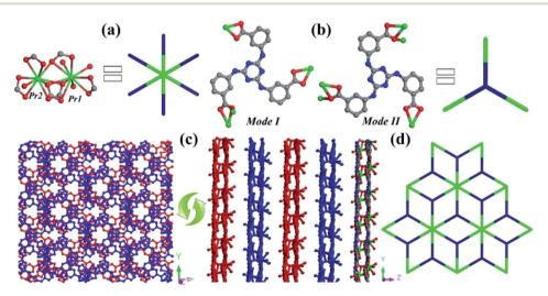
Fig. 1 (a) Binuclear  $\{Pr_2(COO)_6\}$  subunits viewed as 6-connected nodes. (b) Two coordination modes of TATMA<sup>3-</sup> ligands viewed as 3-connected nodes (hydrogen atoms are omitted for clarity and C, gray; O, red; N, blue; and Pr, green) (c) view of the 2D networks packed together in the ABAB fashion. (d) Simplified 2D coordination framework with the Schläfli symbol of  $(4^3)_2(4^6 \cdot 6^6 \cdot 8^3)$ .
