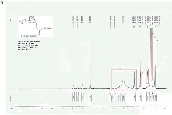
Fig. 2 (A) FTIR spectra of (R2) p-mannose and (R1) O-stearoyl mannose. (B) The <sup>1</sup>H NMR spectra of O-stearoyl mannose.
