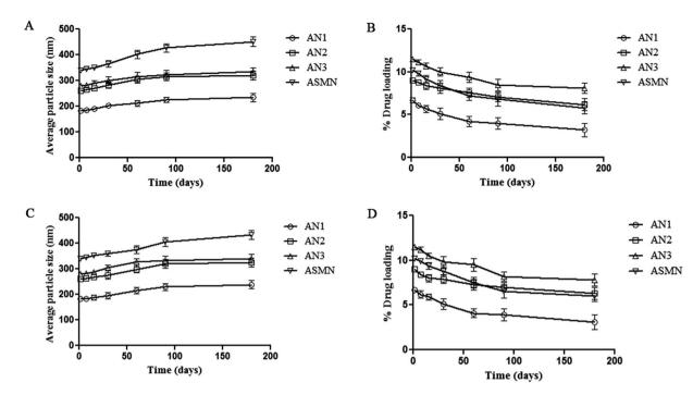
Fig. 8 A storage stability study of the formulated nanoparticles at 4 °C: (A) particle size analysis and (B) % drug loading study, and at room temperature (25 °C): (C) particle size analysis and (D) % drug loading study.
