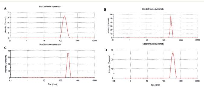
Fig. 5 A particle size distribution study of (A) AN1, (B) AN2, (C) AN3 and (D) ASMN.
