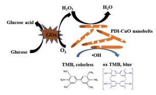
Scheme 1 Schematic illustration of colorimetric sensor for H<sub>2</sub>O<sub>2</sub> and glucose detection using PDI-CuO nanobelts as catalysts
