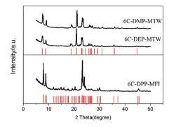
Fig. 1 XRD pattens of 6C-DMP-MTW, 6C-DEP-MTW, 6C-DPP-MFI. The red line represents the characteristic diffraction of zeolite MTW and MFI (from http://www.iza-online.org/).
