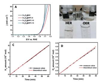
Fig. 5 (A) OER polarization curves for  $\text{Co}_9\text{S}_8$ @NPC-5,  $\text{Co}_9\text{S}_8$ @NPC-10,  $\text{Co}_9\text{S}_8$ @NPC-15 and  $\text{Co}_9\text{S}_8$ @NC electrodes at 10 mV s<sup>-1</sup> in 1.0 M KOH. (B) A photograph of overall water splitting and the gas collection equipment. (C and D) The dependence of the theoretically calculated and experimentally measured hydrogen and oxygen amounts on time during electrocatalytic water splitting using  $\text{Co}_3\text{S}_8$ @NPC-10.
