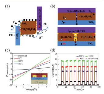
Fig. 7 Schematic diagram of (a) band gap of perovskite, Pbl2 and perovskite device after passivation, (b) electrons and holes transfer process in the pristine and passivated perovskite film. (c) The currentvoltage (I-V) and (d) current-time (I-t) characteristic curves of the perovskite film annealed at different temperatures on the Si substrates under illumination (650 nm,  $1 \text{ mW cm}^{-2}$ ).
