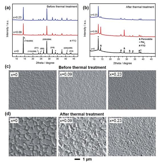
Fig. 2 Structure analysis of perovskite films. (a, b) XRD patterns for  $Cs_xMA_{1-x}Pbl_3$  before and after thermal treatment. (c, d) Top-down view SEM images of perovskite films before and after thermal treatment.
