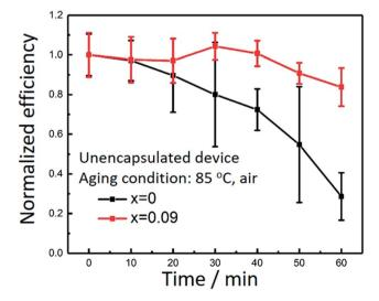
Fig. 5 Thermal stability of assembled perovskite solar cells from Cs doping and undoped perovskite.
