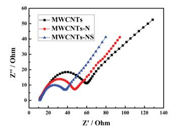
Fig. 4 Electrochemical impedance spectroscopy of glassy carbon electrodes modified by different MWCNTs samples in 1.0 mol  $\rm L^{-1}$  VOSO<sub>4</sub> + 3.0 mol  $\rm L^{-1}$  H<sub>2</sub>SO<sub>4</sub> at open-circuit voltage.
