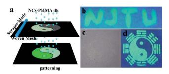
Fig. 6 (a) The schematic of patterning by screen printing. (b), (d) Images ( $\lambda_{ex} = 365$  nm) and (c) (under daylight) of the patterning obtained using the mixture of CsPbBr<sub>3</sub> NC-PMMA.
