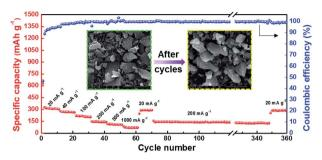
Fig. 8 Discharge capacities of HC-1000 at different current densities of 20, 40, 100, 200, 500 and 1000 mA  $\rm g^{-1}$ , respectively. A long-term cycling performance is recorded from the 70<sup>th</sup> to the 350<sup>th</sup> cycles at 200 mA  $\rm g^{-1}$  and SEM images of the HC-1000 electrodes before and after 360 cycles.
