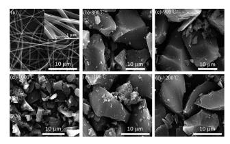
Fig. 1 SEM images of PVP precursors and as-prepared samples at different temperature (a) PVP nanofibers prepared by electrospinning (b) HC-800 (c) HC-900 (d) HC-1000 (e) HC-1100 (f) HC-1200
