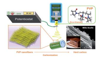
Scheme 2 Schematic illustration of the synthesis process for the mille-feuille shaped hard carbons derived from PVP.
