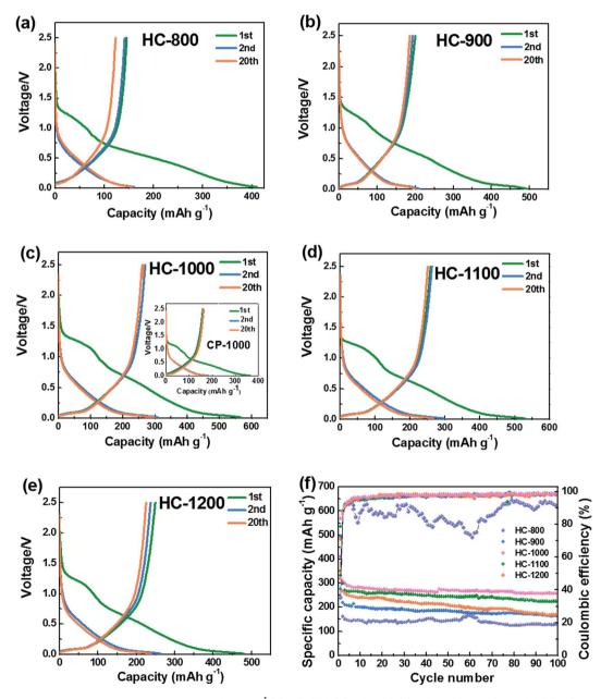
Fig. 5 Discharge-charge profiles of hard carbons at 20 mA g<sup>-1</sup> (a) HC-800 (b) HC-900 (c) HC-1000 and CP-1000 (d) HC-1100, and (e) HC-1200, (f) cycling performance of HC electrodes tested at 20 mA  $\rm g^{-1}$ , the voltage range is between 0.01 and 2.5 V.
