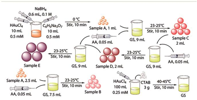
Fig. 1 Schematic illustration for the synthesis procedure of Au NPs with different diameters (CTAB: hexadecyl trimethyl ammonium bromide; AA: ascorbic acid).
