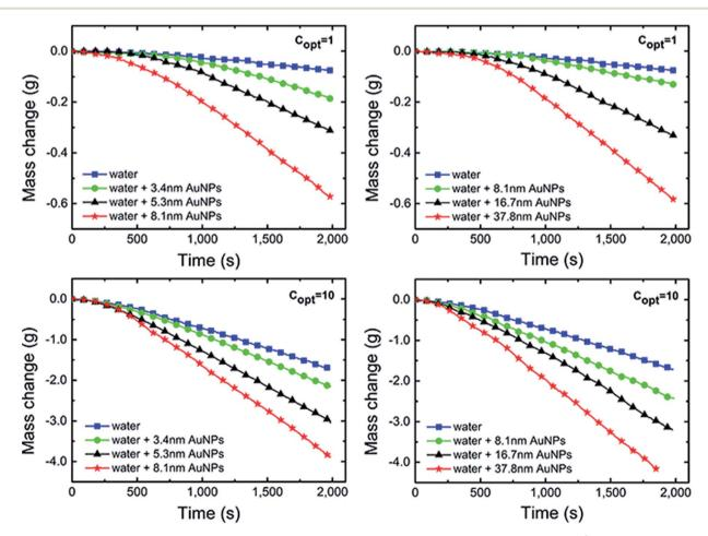
Fig. 5 The mass loss (evaporated water) of Au NPs dispersions with different diameters under 1 and 10 kW  $m^{-2}$  xenon lamp's illumination compared with pure water. Au NPs from G1 (a) and G2 (b) were irradiated under 1 kW  $m^{-2}$  illumination. Similarly, Au NPs from G1 (c) and G2 (d) were irradiated under 10 kW  $m^{-2}$  illumination.
