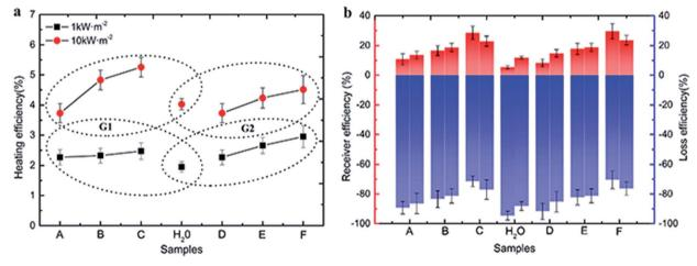
Fig. 8 Three kinds of efficiencies for photothermal conversion. (a) Heating efficiency of Au nanoparticles from G1 and G2 under 1 and 10 kW m $^{-2}$ solar illumination. (b) Receiver efficiency and loss efficiency of Au nanoparticles from G1 and G2 under 1 and 10 kW m<sup>-2</sup> illumination.
