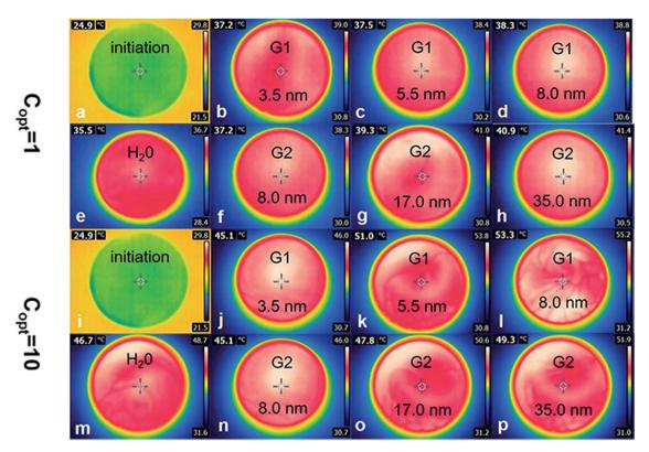
Fig. 7 The temperature of pure water and Au NPs nanofluids with different diameters before and after  $\sim$  2000 s solar illumination under 1 kW m $^{-2}$ (a)-(h) and 10 kW m<sup>-2</sup> solar illumination (i)-(p), respectively.
