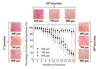
Fig. 2 Relationship between percentage of successful insertions and the number of insertions with MNs with different heights. The microscopic images of porcine skin treated with the MNs at 1<sup>st</sup>, 10<sup>th</sup> and 20<sup>th</sup> insertion are provided on the left, top and right of the graph respectively. Each data point represents the average of 5 experiments. Standard deviation bars are shown.
