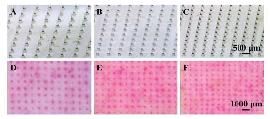
Fig. 4 Microscopic images showing the enlarging structure of the fabricated PLA MNs and the piercing effect of the MNs. (A–C) MN arrays with a height of  $600 \mu m$  and different densities of (A) 144 MNs per cm<sup>2</sup>, (B) 196 MNs per cm<sup>2</sup> and (C) 256 MNs per cm<sup>2</sup>. (D–F) The porcine skin samples treated with MNs with different densities of (D) 144 MNs per cm<sup>2</sup>, (E) 196 MNs per cm<sup>2</sup> and (F) 256 MNs per cm<sup>2</sup>.
