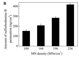
Fig. 3 The amount of sulforhodamine B permeated into the porcine skin treated with MNs with (A) different heights (600, 700 and 800  $\mu$ m) and (B) densities (100, 144, 196 and 256 MNs per cm<sup>2</sup>) in 5 min from 0.1 mg mL<sup>-1</sup> surforhodamine B solution. Each data point represents the average of 5 experiments. Standard deviation bars are shown.
