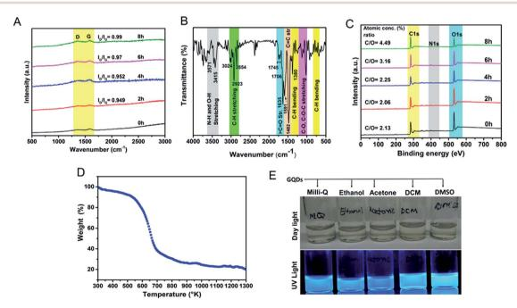
Fig. 4 Physical characterization of GQDs. (A) Raman spectrum recorded at the different hydrothermal reaction, (B) FTIR analysis, and (C) comparative survey XPS analysis showing N-doped characteristics and highly oxygen-rich surface, (D) TGA analysis, and (E) dispersion of GQDs in different solvents (1.0 mg mL $^{-1}$ ).
