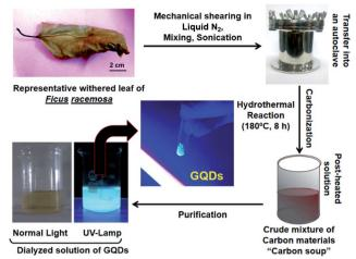
Fig. 1 A general workflow towards synthesis, extraction, and purification of multi-luminescent GQDs from withered leaves of F. racemosa. Withered leaves of F. racemosa crushed in liquid N2 followed by thermal disintegration undergo carbonization in a hydrothermal reaction chamber. The resultant crude mixture is a soup of different types of carbon nanomaterials which was further subjected to purification steps and freeze-drying to attain solid-state GQDs.
