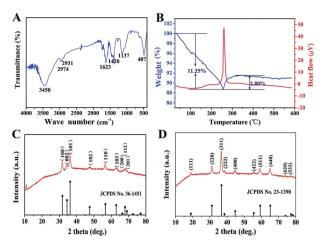
Fig. 1 (A) The FT-IR spectrum of the ZnCo-precursor. (B) The TG and DTA curves obtained for the ZnCo-precursor. (C) The XRD pattern of the ZnCo-precursor. (D) The XRD pattern of  $ZnCo_2O_4$ .
