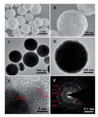
Fig. 2 (A and B) SEM images, (C and D) TEM images, (E) HRTEM image and (F) the corresponding SAED pattern of the  $ZnCo_2O_4$  microspheres.
