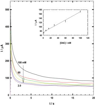
Chronoamperometry diagram for 1 mM DAC in B-R buffer pH 2.
