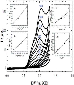
Fig. 6 Cyclic voltammograms (CV) of 1.0 mM DAC at CPE/Cs/CNT-Co in B-R buffer pH 2.0 at: 10, 25, 50, 75, 100, 150, 200 and 300 mV s<sup>-1</sup> Inset (A) plot of the anodic peak current values versus square root of scan rate. Inset (B) plot of log the anodic peak current versus log the scan rate. Inset (C) plot of the anodic peak potential values versus In scan rate. Inset (D) plot of the anodic peak potential values versus scan rate.
