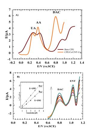
Fig. 9 (A) DPV of B-R buffer solution (pH 2.0) containing DAC with AA and UA monitored at bare CPE and CPE/Cs/CNT-Co. (B) DPV of B-R buffer solution (pH 2.0) containing DAC and ENT by varying their concentrations from 1 to 5 µM at CPE/Cs/CNT-Co. Inset: electrocatalytic peak current versus DAC and ENT concentration.
