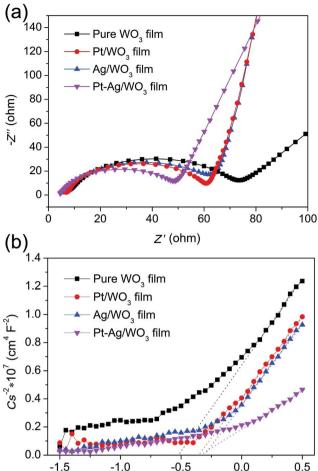
Fig. 9 EIS Nyquist plots (a) and Mott-Schottky plots (b) of the pure WO<sub>3</sub>, Pt/WO<sub>3</sub>, Ag/WO<sub>3</sub>, and Pt-Ag/WO<sub>3</sub> thin-film electrodes.
