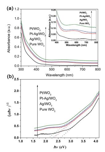
Fig. 6 (a) UV-vis diffuse reflectance absorption spectra of the asprepared samples (the inset shows the region from 400 to 800 nm). (b) Plots of  $(\alpha h v)^{1/2}$  versus photon energy hv of these samples.
