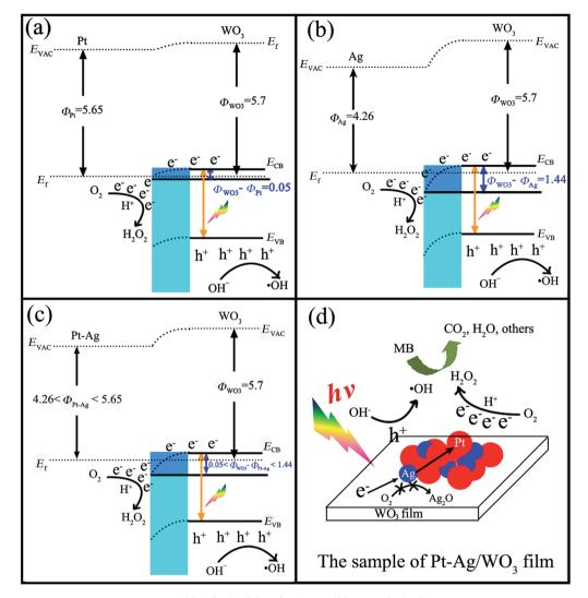
Scheme 2 Schematic energy-band diagrams for (a) Pt/WO<sub>3</sub>, (b) Ag/WO<sub>3</sub>, and (c) Pt-Ag/WO<sub>3</sub> ( $E_{\text{vac}}$ ,  $E_{\text{CB}}$ ,  $E_{\text{VB}}$ ,  $E_{\text{f}}$ ,  $\Phi_{\text{M}}$  and  $\Phi_{\text{WO}_3}$  denote vacuum level, Fermi level, conduction band level, valence band level, work function of metal, and work function of WO<sub>3</sub>, respectively (in eV)). (d) Photocatalytic mechanism for the degradation of MB on the Pt-Ag/WO<sub>3</sub> catalyst.
