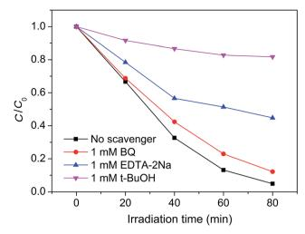
Fig. 10 Plots of photogenerated carrier trapping during the photodegradation of MB by Pt-Ag/WO3 thin film under visible-light irradiation
