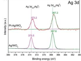
Fig. 5 XPS spectra of (a) W 4f and (b) Pt 4f and (c) Ag 3d high-resolution spectra for the different as-prepared samples.
