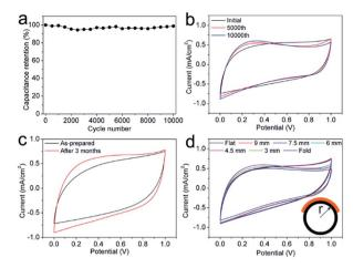
Fig. 5 (a) Cycling stability at a scan rate of 50 mV s<sup>-1</sup>, (b) CV curves of the initial, 5000th, and 10 000th cycles, (c) CV curves of the asprepared C/TiO<sub>2</sub> MSC and the MSC after 3 months (scan rate 50 mV  $s^{-1}$ ), and (d) CV curves of MSCs bent with different curvature radii (scan rate 50 mV s<sup>-1</sup>). Inset in (d) is a schematic picture of a single MSC bent at different curvature radii
