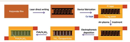
Fig. 1 Schematic illustration for the fabrication of a carbon/TiO<sub>2</sub> micro-supercapacitor with photo-rechargeable capability.
