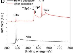
Fig. 3 Raman (a) and XPS spectra (b) of the structures before and after electrophoretic deposition of  $TiO_2$  nanoparticles.
