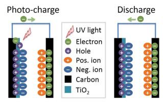
Fig. 7 A schematic illustration of the tentative photo-charge and discharge mechanism.
