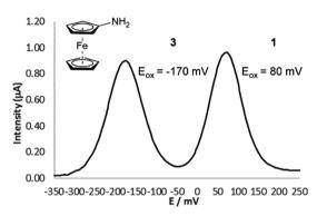
Fig. 1 Differential pulse voltammogram obtained for substrate 1 (0.1 mM) and ferrocenylamine 3 (0.1 mM) in 50 mM pH 7 Tris buffer.
