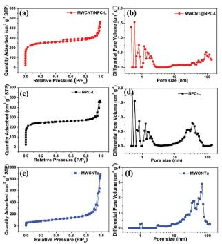
Fig. 5 Nitrogen adsorption-desorption isotherms and pore size distribution: (a) and (b) MWCNT/NPC-L. (c) and (d) NPC-L. (e) and (f)
