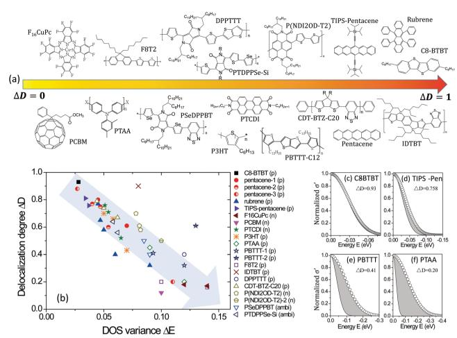
Fig. 5 (a) Schematic representations of materials roughly from a low to high delocalization degree. (b) The values of the delocalization degree  $\Delta D$  and the DOS variance  $\Delta E$  are plotted for different semiconductors. The grey arrow shows the direction of increasing disorder in the charge transport. (c-f) The microscopic conductivity and the DOS for some materials, where the grey areas represent the reduced microscopic conductivity owing to the localization of charge transport.
