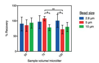
Fig. 3 P-CLIP particle recovery efficiency. Plot of the percentage of particles counted before and after P-CLIP for 2.8  $\mu$ m – (blue) 5  $\mu$ m – (red) and 10  $\mu$ m – (green) diameter magnetic particles from 50, 75, or 100  $\mu$ L volumes of PBS. Error bars represent  $\pm$  1 relative std. dev. (n = 3). \*P  $\leq$  0.05, \*\*P  $\leq$  0.01.
