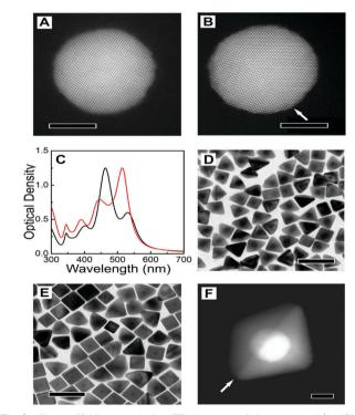
Fig. 2 (A and B) High-resolution TEM images of single-crystal (A, 12NR) and mono-twinned (B, 12NT) seeds. (C) UV-vis spectra of 20NT (red line) and 12NT (black line) seeds coated with silver. (D and E) Representative TEM images of 20NT (D) and 12NT (E) seeds after silver growth. (F) HAADF-STEM image of an Au seed coated with Ag, forming a triangular-base nanobipyramid. The white arrows in (B) and (F) point to the corresponding twin planes. Scale bars: (A and B) 5 nm; (D and E) 100 nm; (F) 10 nm.
