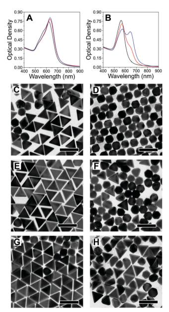
**Fig. 3** (A and B) UV-vis spectra of 20NT (A) and 20NR (B), grown in the presence of different concentrations of iodide: 50 μM (black), 75 μM (red) and 100 μM (blue). (C–H) TEM analysis of 20NT (left) and 20NR (right) grown with different iodide concentrations: 50 μM (C and D), 75 μM (E and F), 100 μM (G and H). Scale bars: 100 nm. (Images at different magnifications are shown in the ESI,† Fig. S12 and S13).
