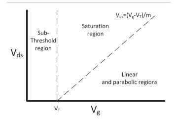
Fig. 2 FET regions of operation. m is the body-effect coefficient ( $m \ge 1$ ). Adapted from figure by Taur and Ning (2013).58
