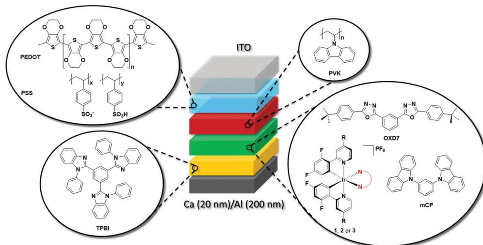
Fig. 10 Schematic for OLED device. The architecture consisted of the following structure: ITO/PEDOT:PSS (40 nm)/PVK (35 nm)/(mCP + active layer + OXD7) (30 nm)/TPBI (60 nm)/Ca (20 nm)/Al (200 nm) structure, where **1**, **2** or **3** act as the active layer.
