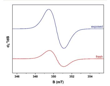
Fig. 2 Comparison of the X-band EPR spectra for the fresh (red) and air-exposed (blue) catalyst recorded at ambient temperature on an aliquot collected after 2 h TOS with 20% MeOH/Ar at a reaction temperature of 260  $^{\circ}$ C.
