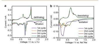
Fig. 3 Cyclic voltammograms of SnSb NCs tested in (a) Li-ion or (b) Na-ion half-cells using a scan rate of  $0.1~\rm mV~s^{-1}$  in the potential range of  $0.005-2.0~\rm V$ .
