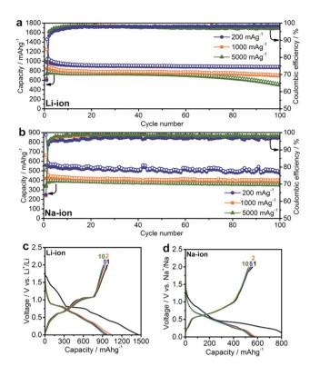
Fig. 2 Electrochemical performance of SnSb NCs. Capacity retention of SnSb NCs in (a) Li-ion and (b) Na-ion half-cells at currents of 200, 1000 and 5000 mA g<sup>-1</sup>. Galvanostatic charge and discharge curves of SnSb NCs in (c) Li-ion and (d) Na-ion half-cells at a current of 200 mA  $g^{-1}$ . All measurements were performed in the potential range of 0.005-2.0 V.
