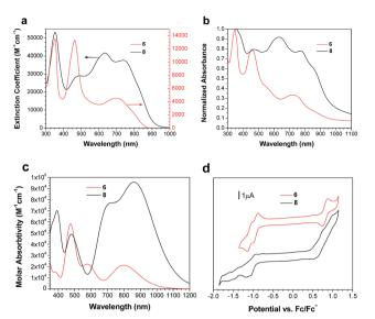
Fig. 2 UV/vis absorption spectra of **6** and **8** in (a) CHCl<sub>3</sub> and (b) as a thin film on glass. (c) theoretical UV/vis spectra of **6** and **8**. (d) Cyclic voltammograms of **6** and **8** in 0.05 mol L<sup>-1</sup> (NBu<sub>4</sub>)PF<sub>6</sub> in CH<sub>2</sub>Cl<sub>2</sub>.
