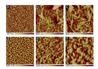
Fig. 4  $10 \times 10$   $\mu$ m AFM images of active layer blends cast from 20 mg mL $^{-1}$  solutions; (a–c) **6**:PC $_{71}$ BM active layers with (a) 0%, (b) 1%, (c) 3% DIO (v/v); (d–f) **8**:PC $_{71}$ BM active layers with (d) 0%, (e) 1%, (f) 3% DIO (v/v).
