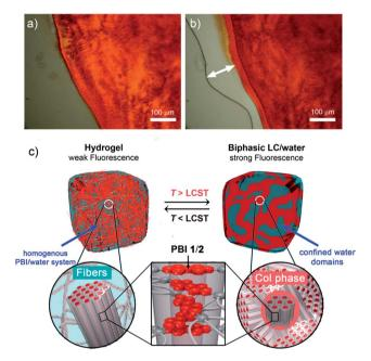
Fig. 5 Optical microscope images of PBI 1 in  $\rm H_2O$  (80 wt% water content) (a) below LCST (40 °C) and (b) above LCST (58 °C). The release of water at the periphery of the gel is indicated with a white arrow. (c) Schematic illustration of the LCST induced phase transition in PBI 1 and PBI 2 hydrogels. Col: columnar nanostructure.
