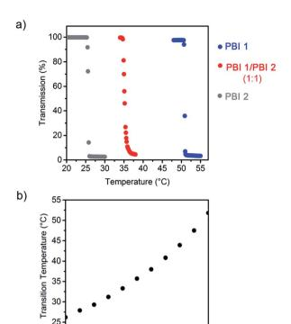
Fig. 2 (a) Transmission at 800 nm of aqueous solutions ( $2.5 \times 10^{-4}$  M) of PBI 1, PBI 2 and PBI 1/PBI 2 (1 : 1) as a function of the temperature. Heating rate  $0.1\,^{\circ}\text{C}$  min $^{-1}$ . (b) Phase transition temperatures for PBI 1/PBI 2 aggregates ( $2.5 \times 10^{-4}$  M) as function of the molar fraction ( $\chi$ ) of PBI 1.
