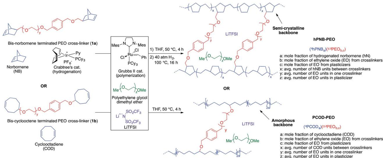
Fig. 2 Hydrogenated polynorbornene–polyethylene oxide (hPNB–PEO) and polycyclooctadiene–polyethylene oxide (PCOD–PEO) cross-linked polymer electrolyte synthesis and nomenclature.
