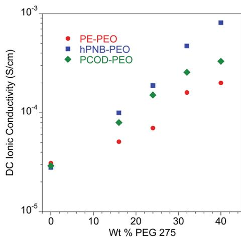
**Fig. 4** Ionic conductivity of plasticized polymer electrolyte as a function of wt% of PEG 275 at 25 °C. All membranes had approximately 80 EO cross-linker units (70 for PE–PEO,<sup>10</sup> 88 for hPNB–PEO, and 75 for PCOD–PEO), [1a] : [NB] or [1b] : [COD] ratios of 1 : 15, and [EO] : [Li] compositions of 20 : 1. Error bars are smaller than the size of the data points. The data for PE–PEO SPEs are from ref. 10.
