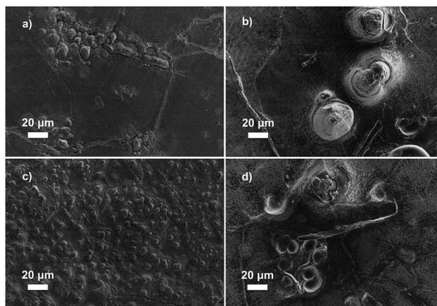
**Fig. 6** Scanning electron microscopy images of a short-circuited Li anode after galvanostatic (a) polarization ( $0.40 \text{ mA cm}^{-2}$ ) and (c) cycling ( $0.26 \text{ mA cm}^{-2}$ ) test with hPNB-PEO electrolyte (plasticized with 32 wt% PEG 275) and (b) polarization ( $0.40 \text{ mA cm}^{-2}$ ) and (d) cycling ( $0.26 \text{ mA cm}^{-2}$ ) test with PCOD-PEO electrolyte (plasticized with 32 wt% PEG 275).
