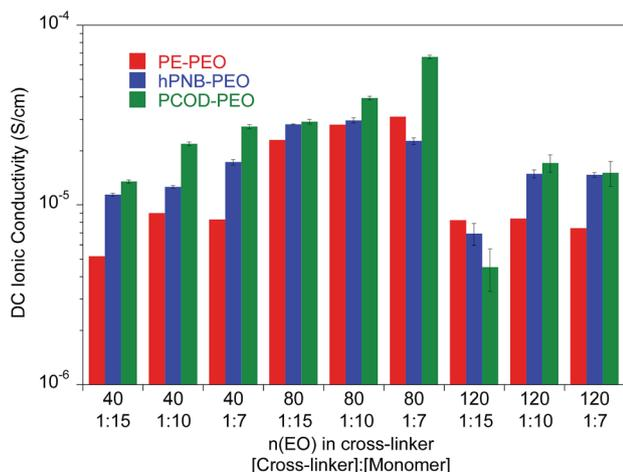
Fig. 3 Ionic conductivity of unplasticized polymer electrolyte with different numbers of ethylene oxide (EO) units in the cross-linker and various [cross-linker] : [monomer] ratios at 25 °C. The data for PE-PEO SPEs are from ref. 10.
