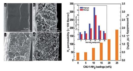
Fig. 14 Left: SEM images of the cross section of pure poly(methyl methacrylate) membrane (a) and MMMs with 5 wt% (b), 15 wt% (c) and 25 wt% (d) CAU-1 loading. Right:  $H_2$  permeability of the MMMs with different CAU-1 loadings and the corresponding  $H_2/CO_2$  selectivities (inset). Reprinted from ref. 95 with permission from Royal Society of Chemistry.
