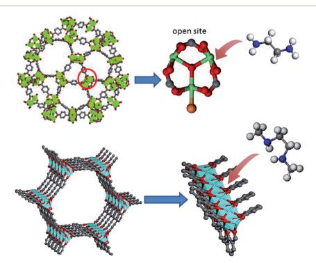
Fig. 4 Schematic route of grafting amines onto the open metal sites of MOFs. Top: MIL-101; bottom: Mg<sub>2</sub>(dobpdc).
