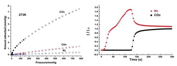
Fig. 7 (Left) Adsorption isotherms for  $CO_2$ ,  $N_2$  and  $CH_4$  at 273 K. (Right) Breakthrough experiment of an equimolar  $CO_2/N_2$  mixture at 0.1 MPa and 273 K. Reprinted from ref. 41 with permission from Royal Society of Chemistry.
