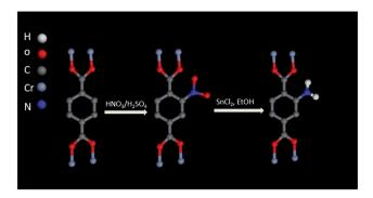
Fig. 3 Representation of the route for preparing NH<sub>2</sub>-MIL-101(Cr) from MIL-101(Cr) *via* PSM.
