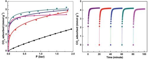
Fig. 9 (Left) CO<sub>2</sub> adsorption isotherms of MIL-101(Cr) before and after PEI loading at 25 °C. Symbol: ■ MIL-101, ● PEI-MIL-101-50, ★ PEI-MIL-101-75, ◆ PEI-MIL-101-100 and ▲ PEI-MIL-101-125. (Right) Cycling CO<sub>2</sub> adsorption kinetics of PEI-MIL-101-100. Reproduced from ref. 62 with permission of Nature Publishing Group.
