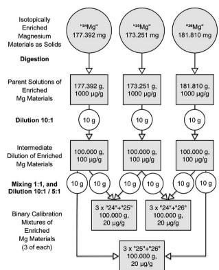
Fig. 7 Dilution and mixing scheme of the second campaign for producing the synthetic isotope mixtures.
