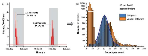
Fig. 6 (a) Representative ICP-MS signal due to two single 10 nm-sized AuNPs ( $C_{\rm NP} = 5 \times 10^5$  NP mL $^{-1}$ ) acquired with the home-built DAQ for 4 ms (counts per 5  $\mu$ s for individual signal pulses identified as individual events). (b) Corresponding intensity histograms of 10 nm-sized AuNPs simultaneously acquired with ICP-MS software (orange) and the home-built DAQ (blue) for 600 s.
