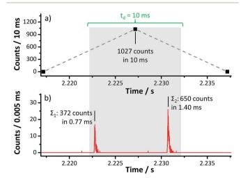
Fig. 4 Transient signal of 30 nm AuNP ( $C_{NP}=2.5\times10^5~\text{NP mL}^{-1}$ ) simultaneously acquired with ICP-MS software (a) and the home-built DAQ (b) for 20 ms. A potential problem in single particle ICP-MS due to particle coincidence within one dwell time is observed in (a) because two individual transient events occurred during one dwell time (grey rectangle indicates a 10 ms dwell time interval used in the ICP-MS software)
