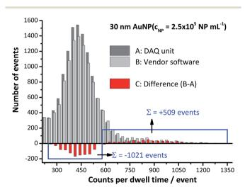
Fig. 3 Differences in the obtained intensity histograms (highlighted in red) of ions originating from 30 nm AuNPs ( $C_{NP} = 2.5 \times 10^5 \text{ NP mL}^{-1}$ ) simultaneously acquired with vendor software (light grey) and the home-built DAQ (dark grey) for 1200 s. With vendor software, significantly fewer events were detected in the expected intensity range, whereas more events with higher signal intensity were observed. This was attributed to possible cases of particle coincidence
