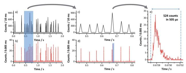
Fig. 1 Representative ICP-MS signal (monitoring  $m/z^{197}$ Au) due to 30 nm AuNPs ( $C_{NP} = 2.5 \times 10^5 \text{ NP mL}^{-1}$ ) acquired simultaneously for 2 s with (a) 10 ms dwell time (vendor software), and (b) 5 µs dwell time (home-built DAQ). First zoom level shows several particle events in (c) and (d) for 500 ms (of highlighted section in a and b). Second zoom level (e) shows the temporal profile of a single particle's ion cloud identified with the home-built DAQ in (d).
