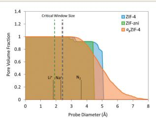
Fig. 3 Pore volume fraction calculated for ZIF-4, ZIF-zni and  $a_q$ ZIF-4 with a range of probe diameters. Dashed lines represent the critical window size for free transport according to the Voronoi representation using Zeo++. 24,25 Note that ZIF-4 undergoes a pressure-induced phase transition, which is not reflected in this scheme
