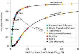
Fig. 4 (a) Comparison of PALS results for a range of materials including polymers, zeolites, MOFs and the present study of ZIF glasses. Only the cavity diameters for the fourth component  $(\tau_4)$  are displayed where multimodal distributions exist. (b) Relative diffusivity predicted from Cohen and Turnbull equation with arbitrary penetrant radii of 0.6 and 1.4 Å. Ref. in Table SI-2 (ESI†).
