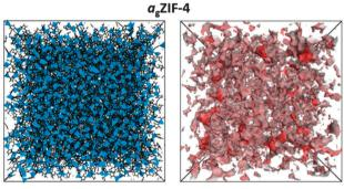
Fig. 1 Structures for ZIF-4 (4  $\times$  4  $\times$  4 supercell, CCDC 602538), ZIF-zni (4  $\times$  4  $\times$  4 supercell, CCDC 120379) and  $a_{\rm q}$ ZIF-4 (2062 Zn atoms). Left: Atomic structures with ligands in black and zinc in blue. Right: Accessible porosity shown as a red Connolly surface, using a probe of 1 Å in diameter.
