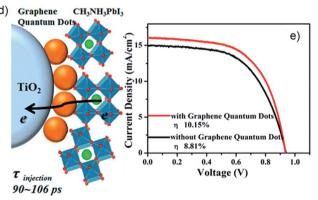
**Fig. 8** (a) Schematic of GQD structure. (b) Energy levels of different layers used in PSCs of Zhu *et al.*,<sup>81</sup> (c) Cross sectional SEM image of PSCs fabricated with GQDs. (d) Schematic illustration of electron generation and injection at the interfaces of TiO<sub>2</sub>, GQDs and perovskites. (e) Current density–voltage curves for the best performing PSCs. Reprinted with permission from ref. 81 © 2014, American Chemical Society.
