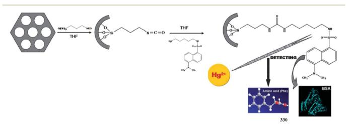
Fig. 290 Schematic of the preparation of nanosensor 330 and its applications for a multifunctional fluorescent probe.
