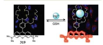
Fig. 281 Chemical structure of RosHg-based fluorescent sensor 319, its proposed binding mode with that of Hg<sup>2+</sup>, and reversibility in the presence of glutathione (GSH).
