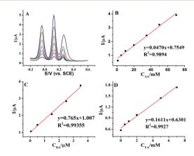
Fig. 5 (A) DPV profiles at AuNPs@MoS $_2$ /GCE in 0.1 M PB solution (pH 7.0) containing different concentrations of AA, DA and UA. From bottom to up the concentrations from 1 mM to 70 mM for AA, 0.01  $\mu$ M to 7  $\mu$ M for DA and 0.01 mM to 12 mM for UA, respectively. (B–D) The plots of the oxidative peak currents *versus* the concentrations of AA, DA and UA.
