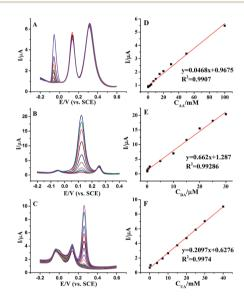
Fig. 4 DPV profiles at AuNPs@MoS $_2$ /GCE in 0.1 M PB solution (pH 7.0) (A) containing 6  $\mu$ M DA, 30 mM UA and different concentrations of AA from 0.05 mM to 100 mM, (B) containing 12 mM AA, 10 mM UA and different concentrations of DA from 0.05  $\mu$ M to 30  $\mu$ M, and (C) containing 50 mM AA, 4  $\mu$ M DA and different concentrations of UA from 0.05 mM to 50 mM. (D–F) The plots of the oxidative peak currents versus the concentrations of AA, DA and UA.
