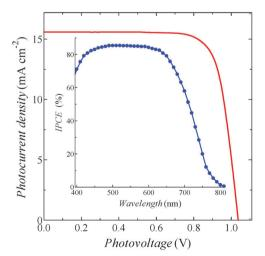
Fig. 3 Typical I-V properties of the ADEKA-1-sensitized solar cell with the highest efficiency of 12.5% (entry 8 in Table 1) under the simulated one sun irradiation (AM-1.5G, 100 mW cm<sup>-2</sup>). Inset shows the IPCE spectrum of the cell.
