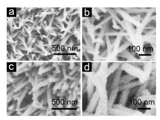
Fig. 2 FESEM images of (a, b) NiCo<sub>2</sub>O<sub>4</sub> NW arrays and (c, d) hierarchical NiCo<sub>2</sub>O<sub>4</sub>@MnO<sub>2</sub> core–shell heterostructured NW arrays grown on Ni foam.
