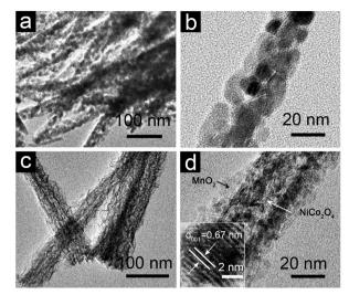
Fig. 3 TEM images of (a, b) NiCo<sub>2</sub>O<sub>4</sub> NWs and (c, d) NiCo<sub>2</sub>O<sub>4</sub>@MnO<sub>2</sub> core-shell heterostructured NWs scratched from Ni foam. The inset of (d) shows a HRTEM image of MnO2 nanoflakes.
