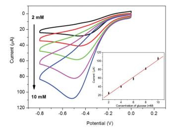
Fig. 5 Cyclic voltammograms of chitosan/GOD/AgNPs-G/GCE in  $\rm O_2$  saturated 0.2 M PBS at pH 7.4 in various concentrations of glucose. Inset is the calibration curves corresponding to amperometric responses at  $\rm -0.5~V$ .
