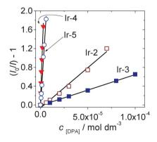
**Fig. 21** Stern–Volmer plots generated from phosphorescence intensity quenching of complex **Ir-2** ( $\lambda_{\rm ex} = 386$  nm), **Ir-3** ( $\lambda_{\rm ex} = 410$  nm), **Ir-4** ( $\lambda_{\rm ex} = 475$  nm) and **Ir-5** ( $\lambda_{\rm ex} = 425$  nm). Phosphorescence was measured as a function of DPA concentration in CH<sub>3</sub>CN.  $1.0 \times 10^{-5}$  mol dm<sup>-3</sup>. 20 °C. Reproduced with permission from ref. 45b.
