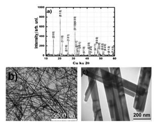
Fig. 1 (a) XRD pattern and (b, c) TEM images of the  $V_2O_5$  nanowires used for the Al-ion secondary battery cathode.
