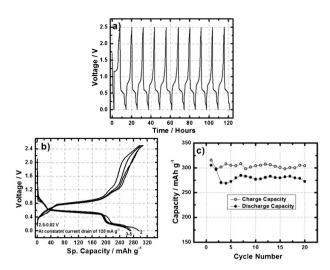
**Fig. 3** (a) Voltage vs. time (b) voltage vs. sp. capacity and (c) cycle life plot of Al-ion battery containing aluminium anode,  $V_2O_5$  nano-wire cathode in ionic liquid under the potential window 2.5–0.02 V and at a constant current drain of 125 mA g<sup>-1</sup>.
