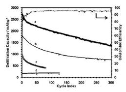
**Fig. 5** Delithiation capacity of: (a) SG paper sample 2, 61 wt% Si, shown with coulombic efficiencies; (b) SG paper sample 1, 59 wt% Si, tested using the CCCV method (sample 1: 1.5–0.005 V, 1000–80 mA g<sup>-1</sup>; sample 2: 1.5–0.02 V, 1000–50 mA g<sup>-1</sup>); (c) SG paper sample 1, crushed and mixed with PVDF binder, cycled at 100 mA g<sup>-1</sup> constant current mode (2.0–0.02 V); (d) graphene-only sample cycled using CCCV method.
