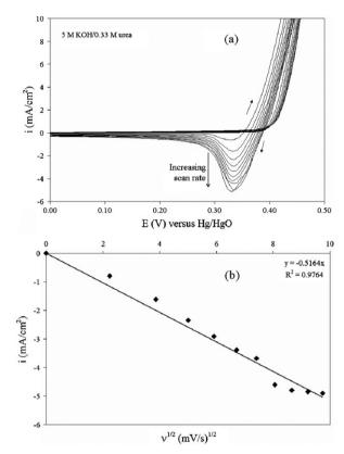
**Fig. 3** (a) Cyclic voltammograms obtained in 5 M KOH  $\pm$  0.33 M urea for the NOMN electrode with various scan rates ( $\nu$ ) from 5 mV s<sup>-1</sup> to 95 mV s<sup>-1</sup>. (b) The plot of cathodic current density variation with  $\nu^{1/2}$ .
