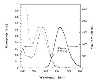
**Fig. 2** Absorption (---) and emission spectra (—) of the D5 dye in MeCN compared with the absorption spectrum of the dye attached to  $\text{TiO}_2$  (···). The excitation wavelength for emission was 460 nm. The absorption and emission maxima in MeCN are 476 nm and 625 nm giving a Stokes shift of 0.62 eV and a zeroth–zeroth transition  $\Delta E_{0-0} = 2.25$  eV. The absorption maximum of the dye attached to the  $\text{TiO}_2$  nanoparticles is blue shifted to 444 nm.
