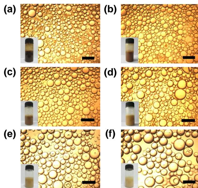
**Fig. 2.** OM images and photos of Pickering emulsions with different lignin content. (a) 1.0 wt.%, (b) 0.5 wt.%, (c) 0.3 wt.%, (d) 0.1 wt.%, (e) 0.05 wt.%, (f) 0.01 wt.%. All scale bars are 200 μm.
