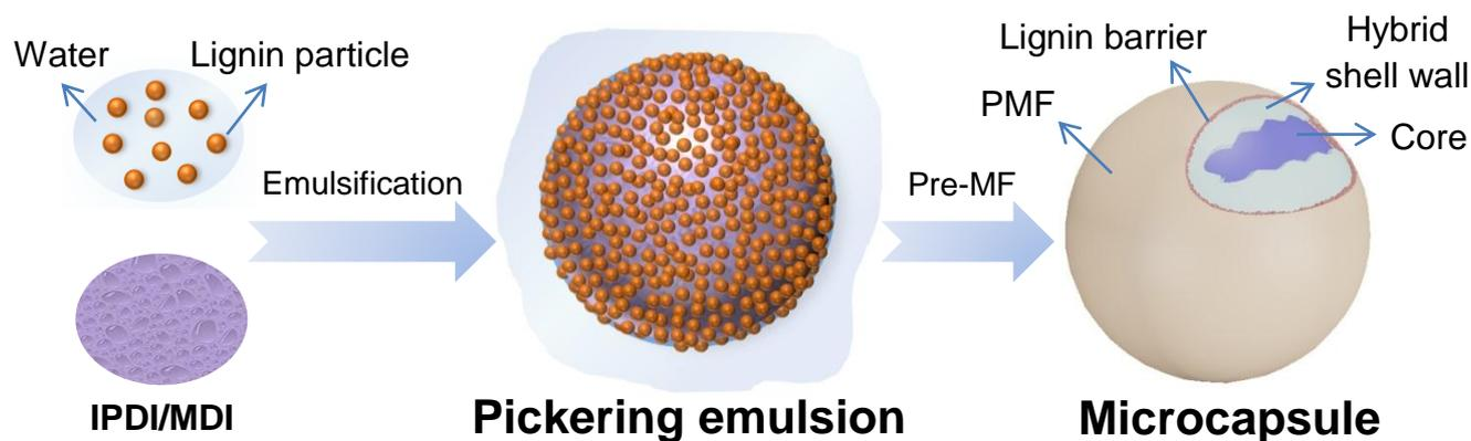
Fig. 1. Schematic for the synthesis process of multilayer composite microcapsules loaded with healing agents based on Pickering emulsion templates.
