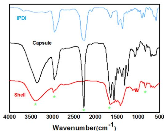
Fig. 6. FTIR spectra of IPDI, the IPDI-containing microcapsule and its shell.
