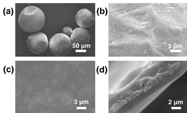
**Fig. 3.** SEM images of IPDI-loading composite multilayer microcapsules (Sample 3). (a) Spherical shaped microcapsule, morphology of (b) outer surface and (c) inner surface, (d) cross section of shell.
