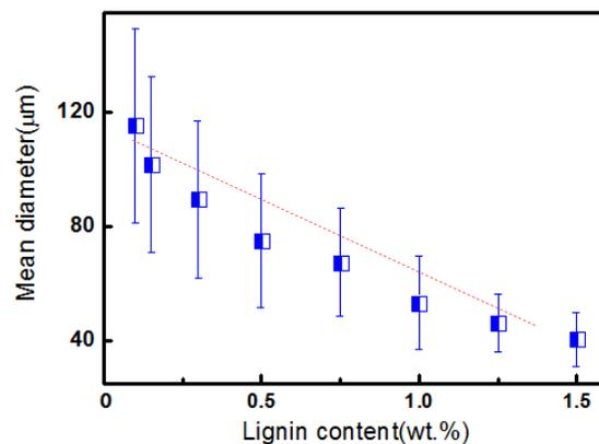
**Fig. 5.** Decrease in mean diameter of microcapsules with increasing amount of lignin contents in Pickering emulsion template.
