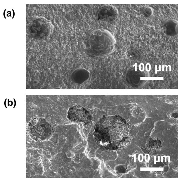
**Fig. 9.** SEM images of (a) fracture surface rinsed with acetone instantly after flawed, and (b) fracture surface revealed on self-healing coating after self-healed.
