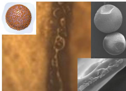
Multilayer composite microcapsules with IPDI prepared from lignin-stabilized Pickering emulsions were used for self-healing epoxy coatings.
