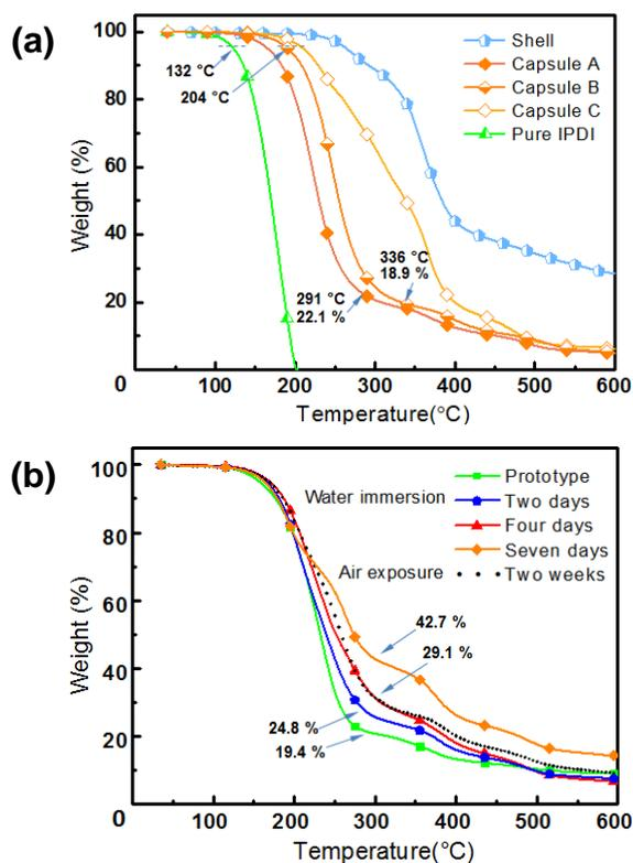
Fig. 7. Characterization of resistant property. (a) TGA curves of IPDI, shell and microcapsules synthesised by Pickering templates with different lignin contents. (A) 0.1 wt.% (B) 0.5 wt.% (C) 2.0 wt.%. (b) TGA curves of microcapsules after immersed in aqueous solution for two days (blue), four days (red), seven days (orange) and exposed in air for two weeks (dotted line). Microcapsules prototype (green) were synthesised from Pickering emulsion template sample 3 (Table 1).
