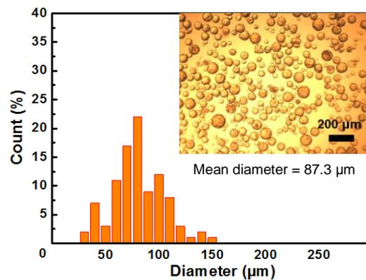
**Fig. 4.** Mean diameter, size distribution and OM image of microcapsules. The microcapsules were prepared by Pickering emulsion template sample 3.
