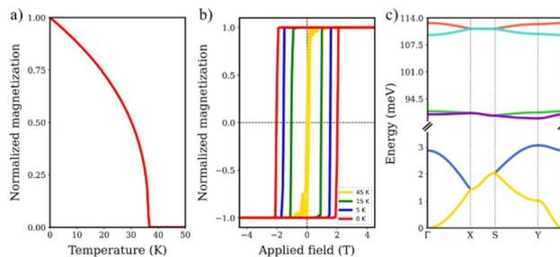
Fig. 4 Simulated (a) Curie temperature, (b) hysteresis loop at different temperatures and (c) magnon dispersion for the  $V_3N@C_{80}$  graphendofullerene network.
