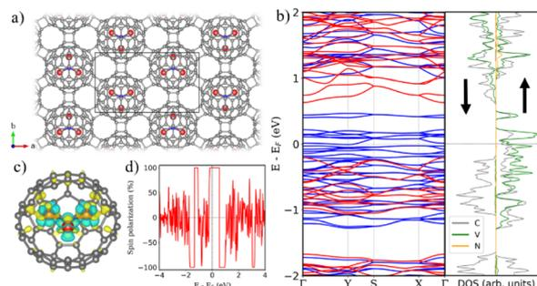
**Fig. 1** (a)  $V_3N@C_{80}$  graphendofullerene top view. Color code: carbon (grey), vanadium (red) and nitrogen (blue). (b) Electronic band structure (left) and projected density of states (PDOS) (right) for the  $V_3N@C_{80}$  monolayer. Blue (red) color in (a) represents spin up (down) electrons. (c) Charge density difference after  $V_3N$  encapsulation. Yellow (blue) regions represent charge accumulation (depletion). (d) Energy level polarization of  $C_{80}$ .
